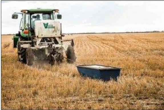
*The researchers hooked together the Veris MSP3 and EM38-MK2, pulling the two soil sensors across each field at the same time to compare the data. Photo by Farming Smarter.*
