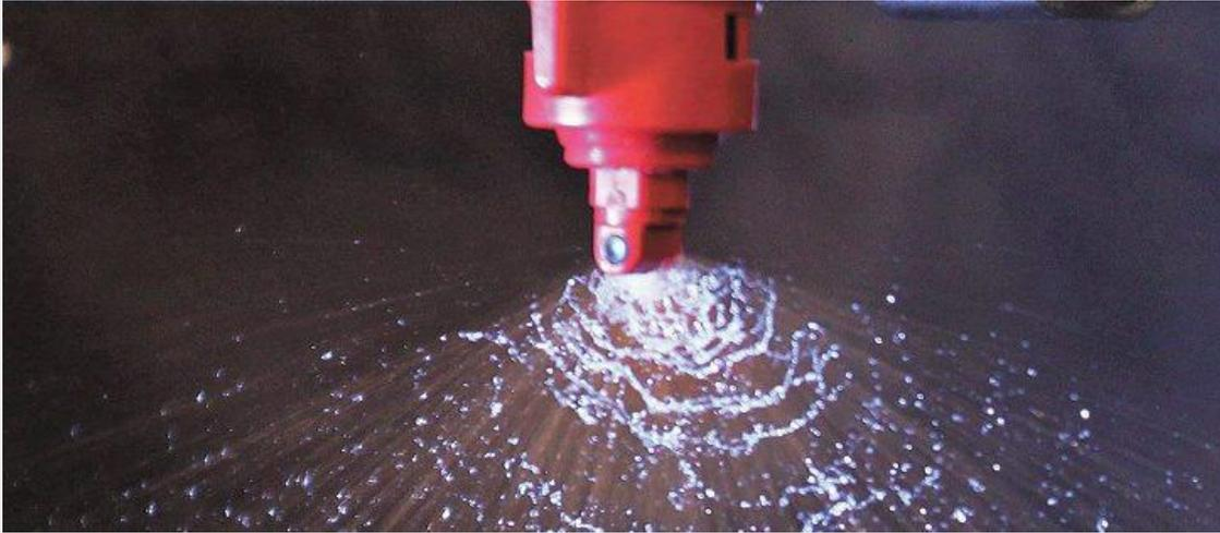
A coarse sprayer nozzle reduces the number of fine droplets. | File photo
