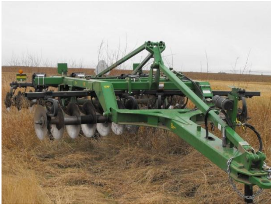
Figures 20 and 21. Field disc cultivator used to incorporate Contans
