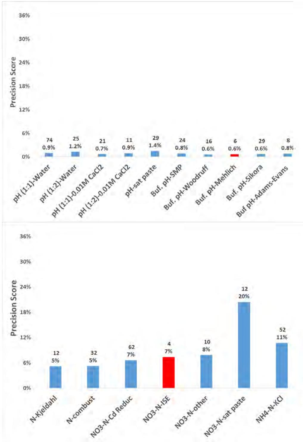
**Fig. 1. Precision scores for various soil pH (top) and nitrogen (N) (bottom) analyses calculated from 43 samples tested by participating NAPT laboratories with the median absolute deviation (MAD) divided by the median for each and then averaged for each analyte. Value above the percentage listed at the top of each bar is the number of labs that submitted data for each analyte (those in red signify too few labs to generate statistics within the NAPT program).**
