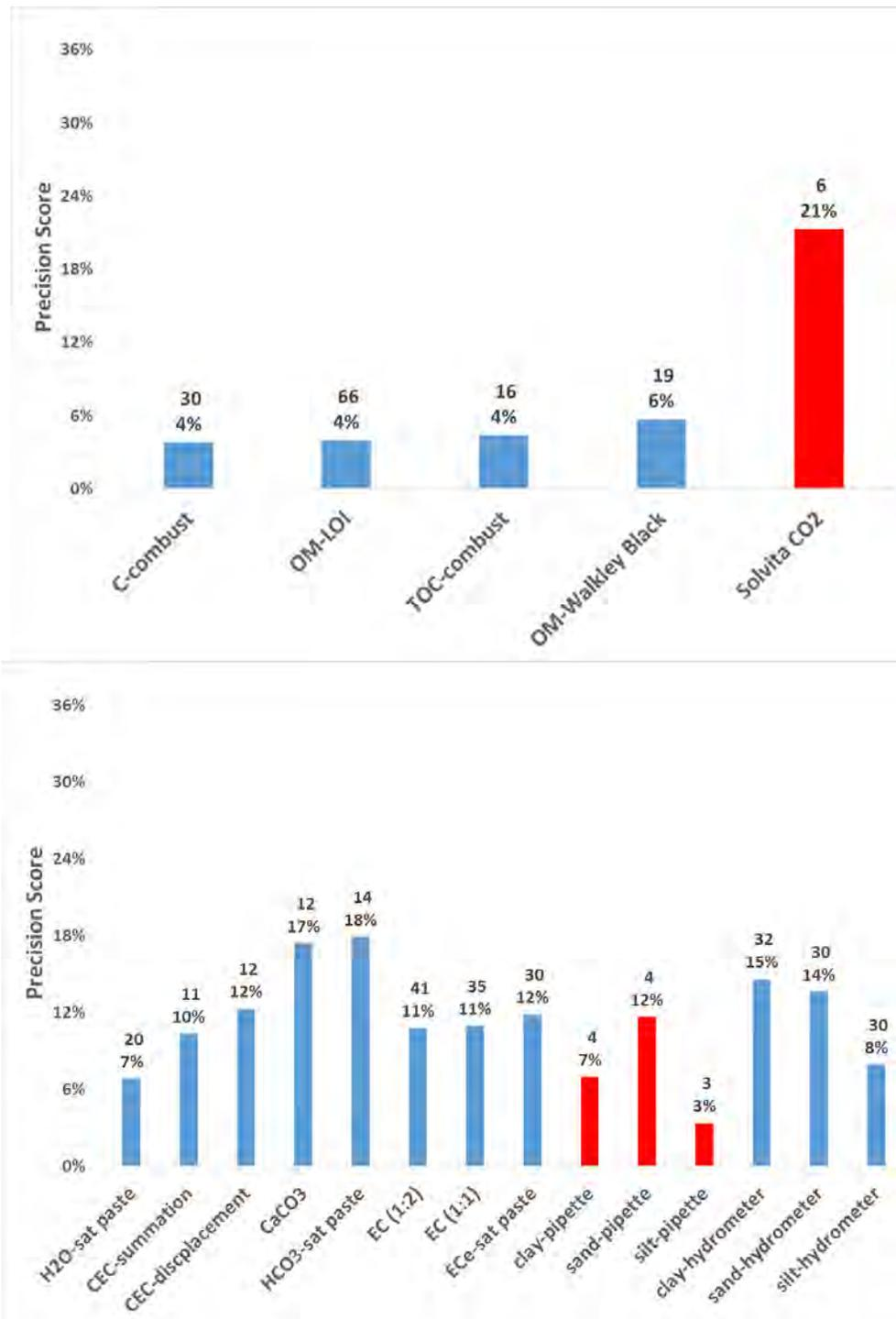
**Fig. 4. Precision scores for various soil carbon related measures (top) and miscellaneous (bottom) analyses calculated from 43 samples tested by participating NAPT laboratories with the median absolute deviation (MAD) divided by the median for each and then averaged for each analyte. Value above the percentage listed at the top of each bar is the number of labs that submitted data for each analyte (those in red signify too few labs to generate statistics within the NAPT program).**
