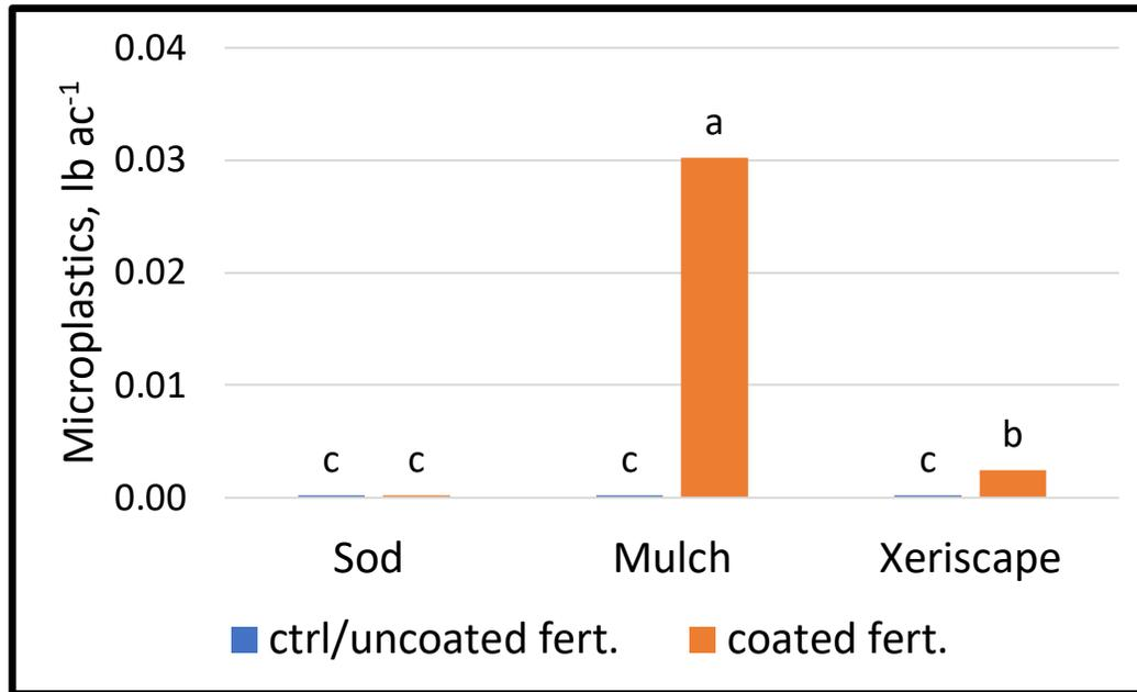
**Fig. 2. Microplastics in runoff water for three urban landscape systems with polymer coated urea (PCU) compared to uncoated control. Bars sharing the same letters on top are statistically identical to one another ( $P < 0.001$ ).**
