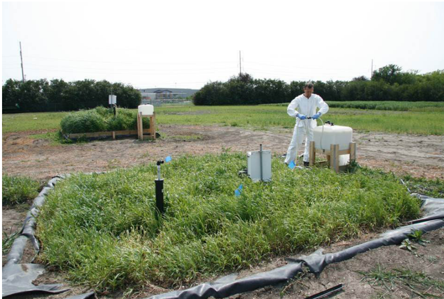
Figure 9. Plants growing on top of a biobed remove water through evapotranspiration and can support microbial growth (photo courtesy Tom Wolf, Agrimetrix Research & Training).
