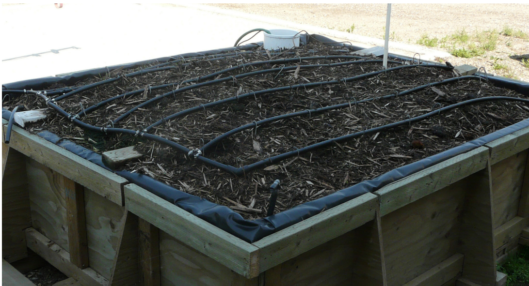
Figure 10. Rinsate is applied uniformly to the biobed through drip tubes laid on top of biomix layer.
