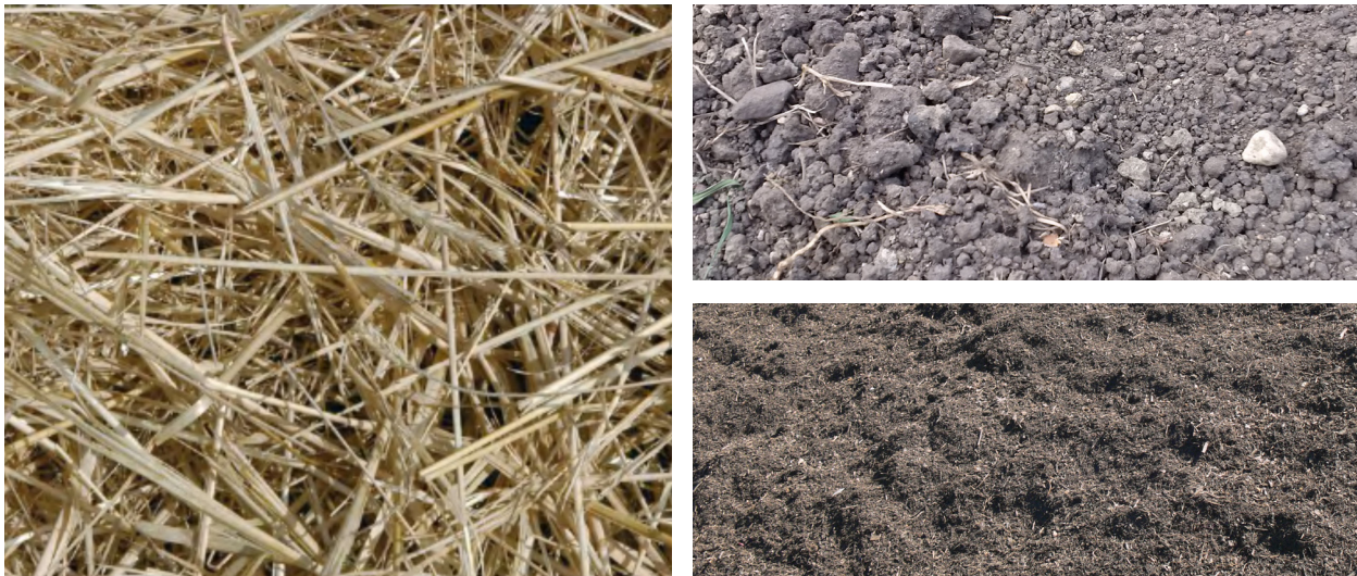
Figure 5. Biomix components [Two parts straw (left) + one part soil (top right) + one part compost (bottom right)] Photo credits - straw: cc by Miquel Pujol Palol; soil: AAFC; compost: cc by C.K. Gurney
