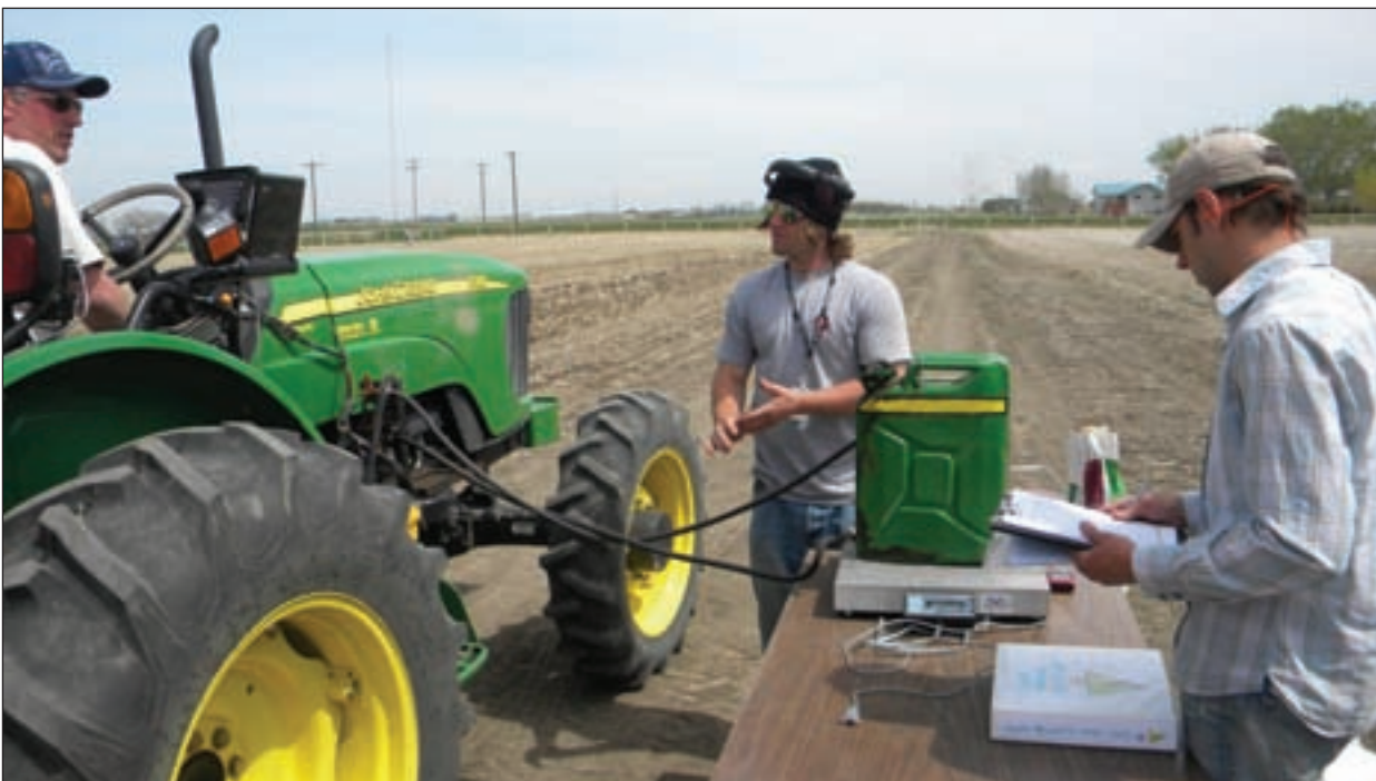
Michael Gretzinger and Brent Nicol weigh the fuel tank between seeding plots as Ken Coles watches from the tractor. PHOTO: TL
