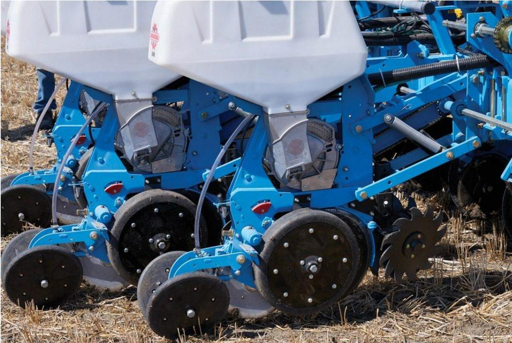
*Seed rows were set at 12- and 20-inch spacing, canola disks were installed and the machine was calibrated for canola seed.*
