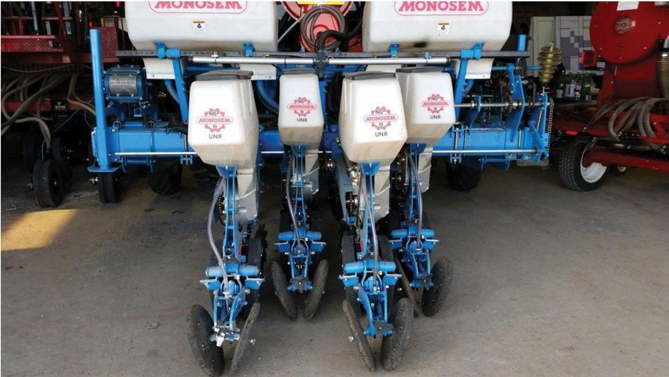
The Monosem is a high precision seeder meant for precise seed placement in both depth and spacing within the row.
