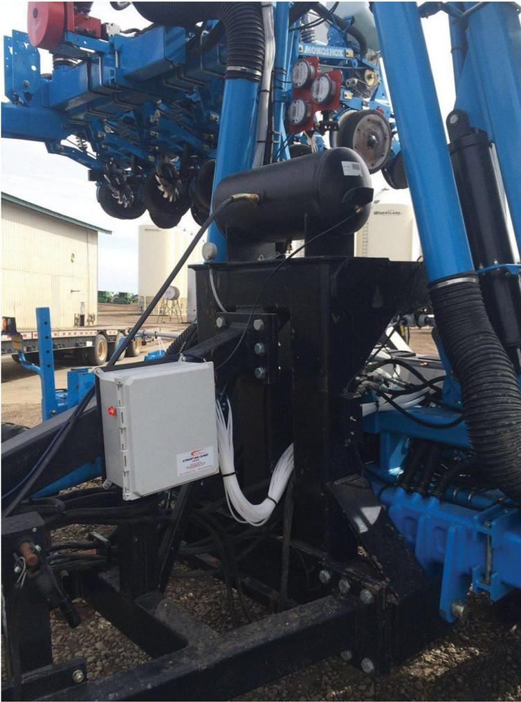
*The Crop Guard Air Box system helps keep the seed metering disk free from plugging.
