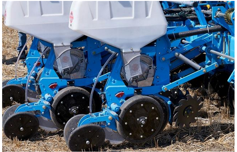
The Monosem planter utilized fixed residue managers but floating residue managers might have improved no-till germination. Irrigated corn has been a mainstay in southern Alberta. Photo: Farming Smarter
