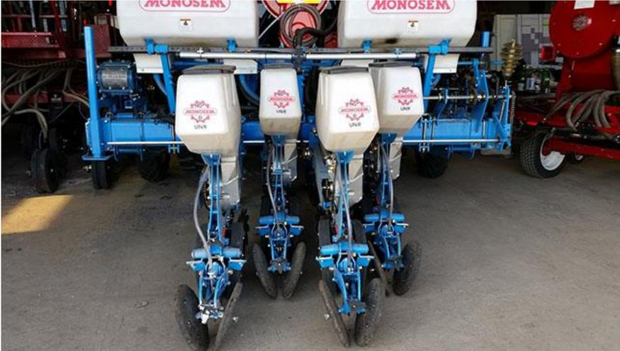
*The Monosem planter set up for no-till seeding provided some advantages over a conventional air drill. Photos courtesy of Farming Smarter*
