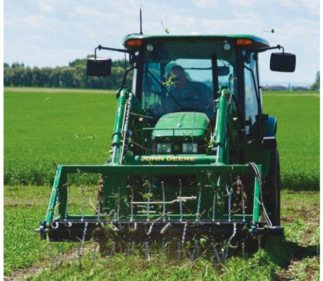
Farming Smarter general manager Ken Coles operates a hail simulator designed to test the effects of “rescue products” for recovering from hail damage. Photo: Farming Smarter
